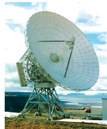
EISCAT Svalbard Radar antenna. The effect of gaps between the panels can be predicted by GRASP9
